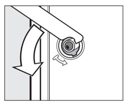
■ Turn the left shipping strut counterclockwise 90° with the enclosed combination wrench.
